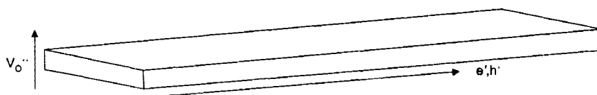
Figure 1. A pattern with a high aspect ratio offers a greatly reduced transport pathway for vacancies compared to that for electronic species.
